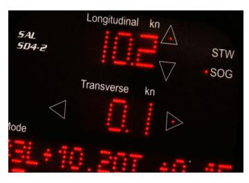
**Display options.** In addition to the speed log displays installed as standard, SAL T200 offers the possibility to add docking log displays, analog displays, and more.
