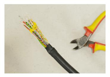
**Easier cable handling.** Low-power digital signals to and from the transducer means the cable does not interfere, and that it may be cut or extended with a junction box without decreased performance. Thus enabling easier and faster cabling work.
