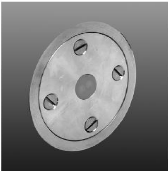
MSSBSV L flush with the hull and TRU properly seated in the guide ring
